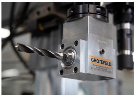
gfnd2101\_b3: Winkelbohrkopf G06-1.1-B an Bohreinheit B50
